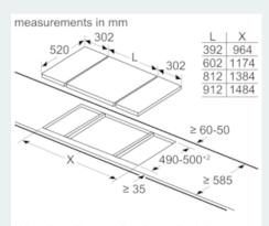
When installing two Domino units right next to a hob, two assembly kits (HZ394301) are required.
